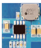
BD9D321EFJ PCB 17mm×20mm=340mm 2
